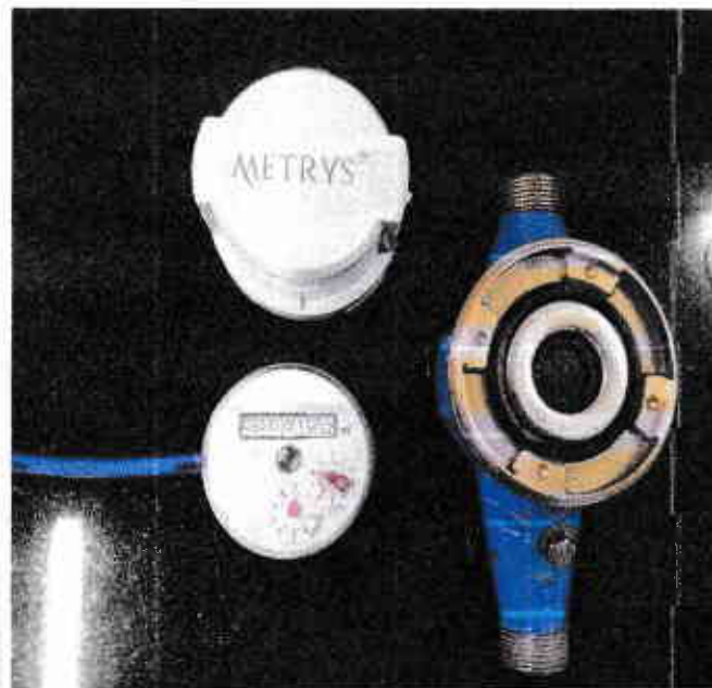
Figure E: DUT After IP 6X test (Open Condition)
