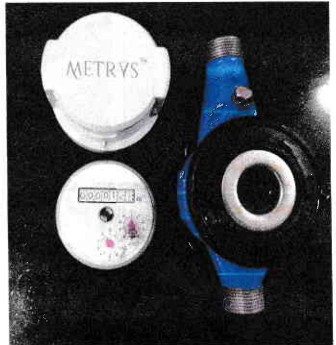
Figure B: DUT After IP X8 test(Open Condition)
